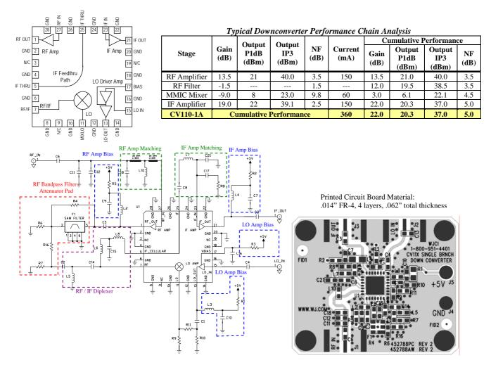
**CV110-1A**: The application circuit can be broken up into four main functions as denoted in the colored dotted areas above: RF/IF diplexing (purple), amplifier matching (green), filtering (red), and dc biasing (blue). There are various placeholders for chip components in the circuit schematic so that a common PCB can be used for all WJ single-branch converters. Additional placeholders for other optional functions such as filtering are also included.
